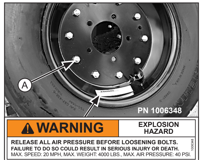
Figure 21. Split Rim Tire Servicing
