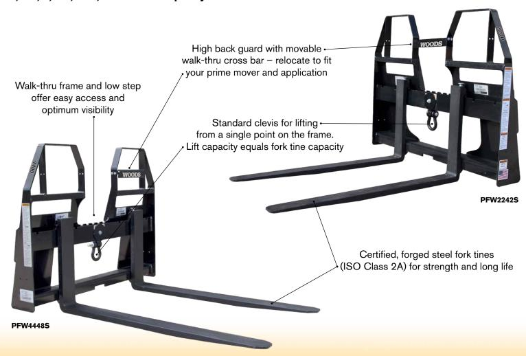
Robotically welded for consistent high quality. Compatible with Skid Steer (ISO 24410), John Deere<sup>®</sup>, and ISO 23206 Quick Attach Systems. Learn more about Woods Loader and Skid Steer attachments at woodsequipment.com.
