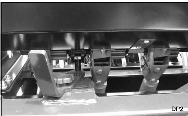
Figure 12. Primary Seed Rate Adjustment Lever
