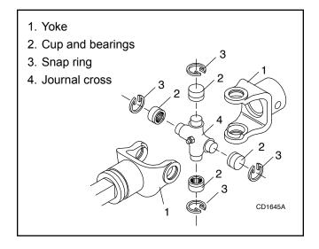
Figure 26. U-Joint Exploded View
