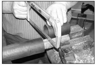
Figure 12. Cut Shaft to Length
