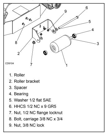
Figure 34. Front Roller Installation
