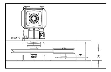
Figure 25. Drive Sheave Installation
