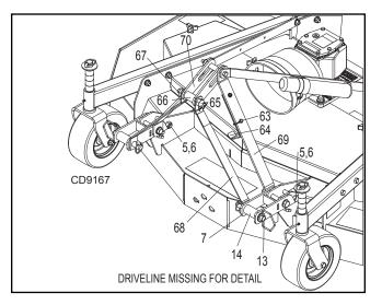
Figure 4. Hitch Assembly
