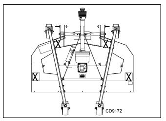
Figure 15. Jackstand Placement
