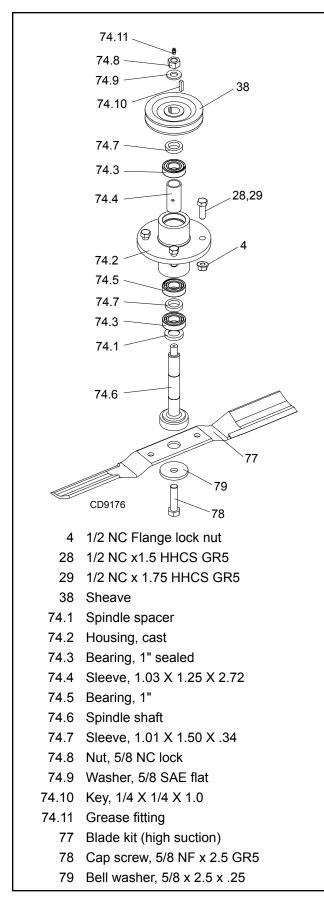
Figure 21. Spindle Assembly
