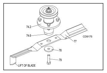
Figure 19. Blade and Spindle Assembly
