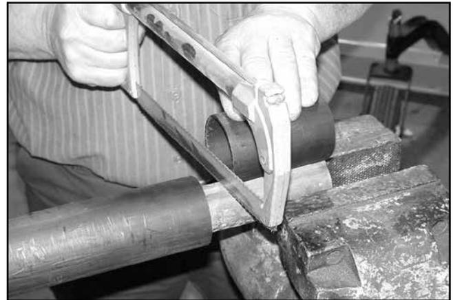
**Figure 12.** Cut Shaft to Length
