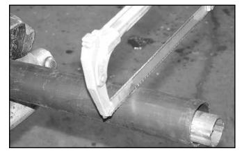
Figure 11. Cut Shield
