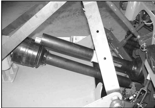
**Figure 9.** Drive Halves Placed Parallel
