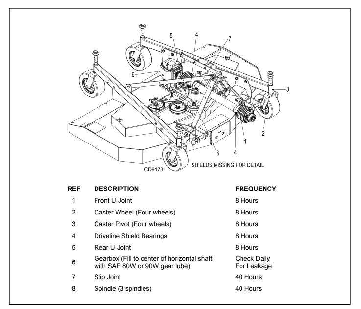
Figure 16. Lubrication Points
