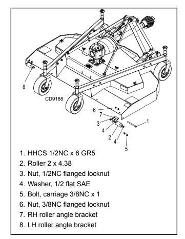
Figure 35. Rear Anti-Scalp Roller Installation
