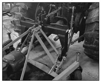
Figure 5. Quick Hitch Attachment
