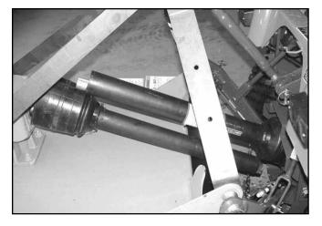
Figure 9. Drive Halves Placed Parallel
