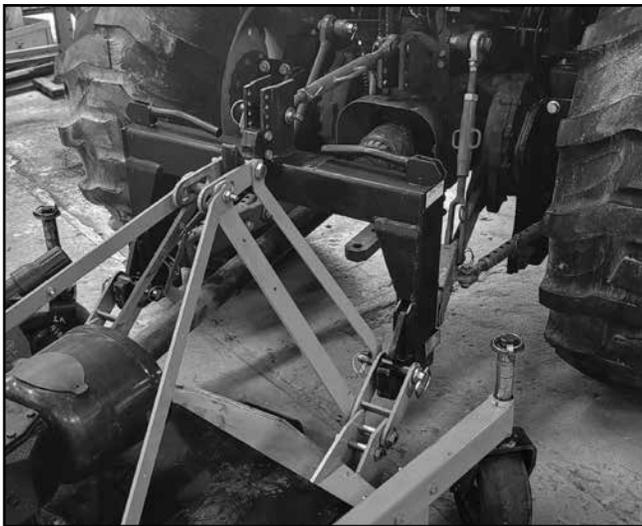
**Figure 5. Quick Hitch Attachment**
