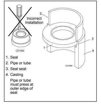
Figure 22. Seal Installation
