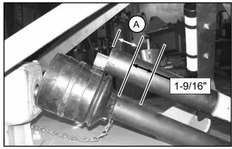
Figure 10. Determine Shield Length
