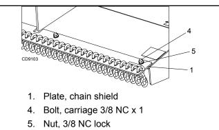
Figure 33. Chain Shielding Installed
