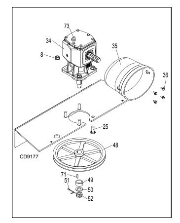
Figure 23. Gearbox Stand Assembly
