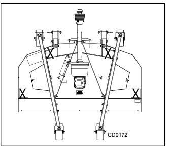
Figure 20. Jackstand Placement
