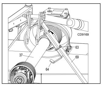
Figure 6. Driveline Holder Storage Position
