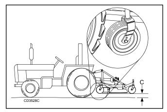
Figure 8. Front Caster Wheel Interference Check
