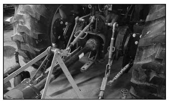
Figure 3. Attach Mower to Tractor
