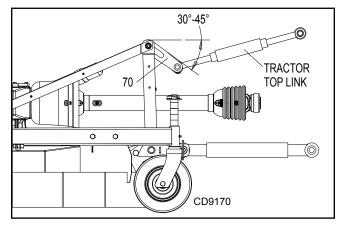
Figure 13. Top Link Adjustment
