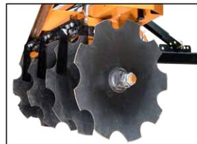
Adjustable disc blades that will cut into and work the soil. Easily adjust the blade angles to till more aggressively depending upon soil conditions.
