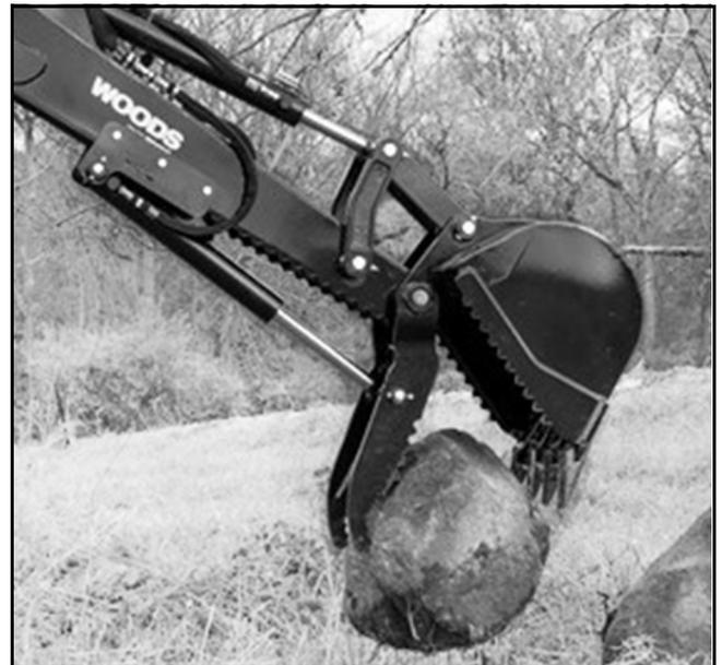
**Figure 12.** Thumb Operation
