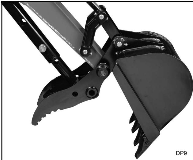
**Figure 31.** Mechanical Thumb Installed
