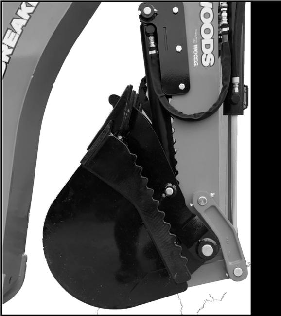
Figure 13. Thumb Storage Position
