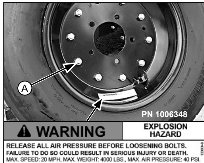
Figure 10. Split Rim Tire Servicing
