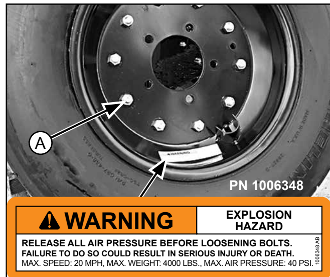
Figure 22. Split Rim Tire Servicing
