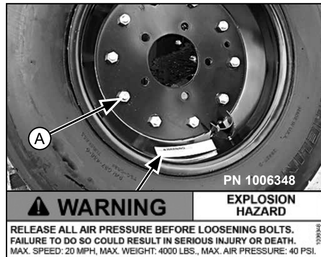
Figure 22. Split Rim Tire Servicing
