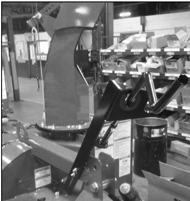
Figure 19. Hand Crank Installed (Alternate Bracket Location)
