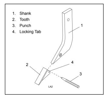
Figure 6. Scarifier Point Replacement
