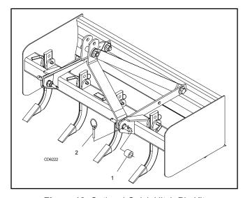
Figure 12. Optional Quick Hitch Pin Kit
