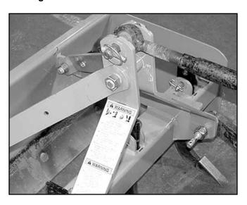
Figure 2. Top Link Connected
