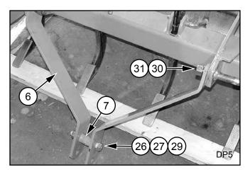
Figure 10. A-frame Bars Assembled
