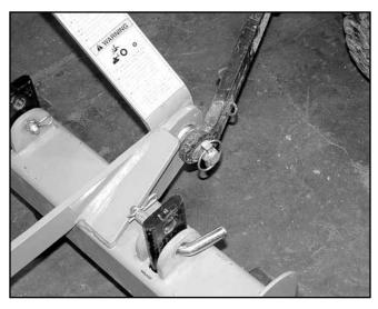
Figure 1. 3-Point Lower Lift Arms Connected
