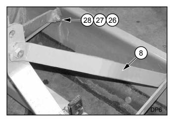
Figure 11. A-frame Support Bars Assembled to A-frame Bars
