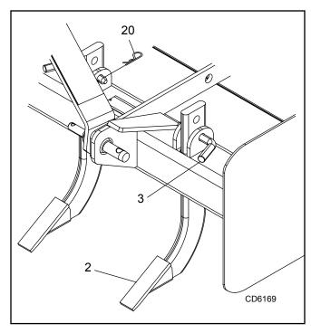
Figure 5. Scarifier Shanks Installed
