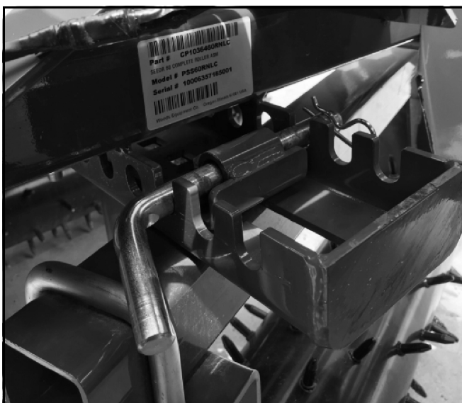
Figure 14. Bent Pin Installation
