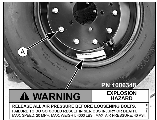
Figure 34. Split Rim Tire Servicing
