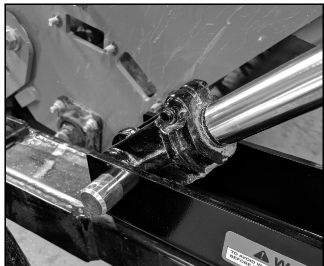
Figure 35. Cylinder Rod End Installed
