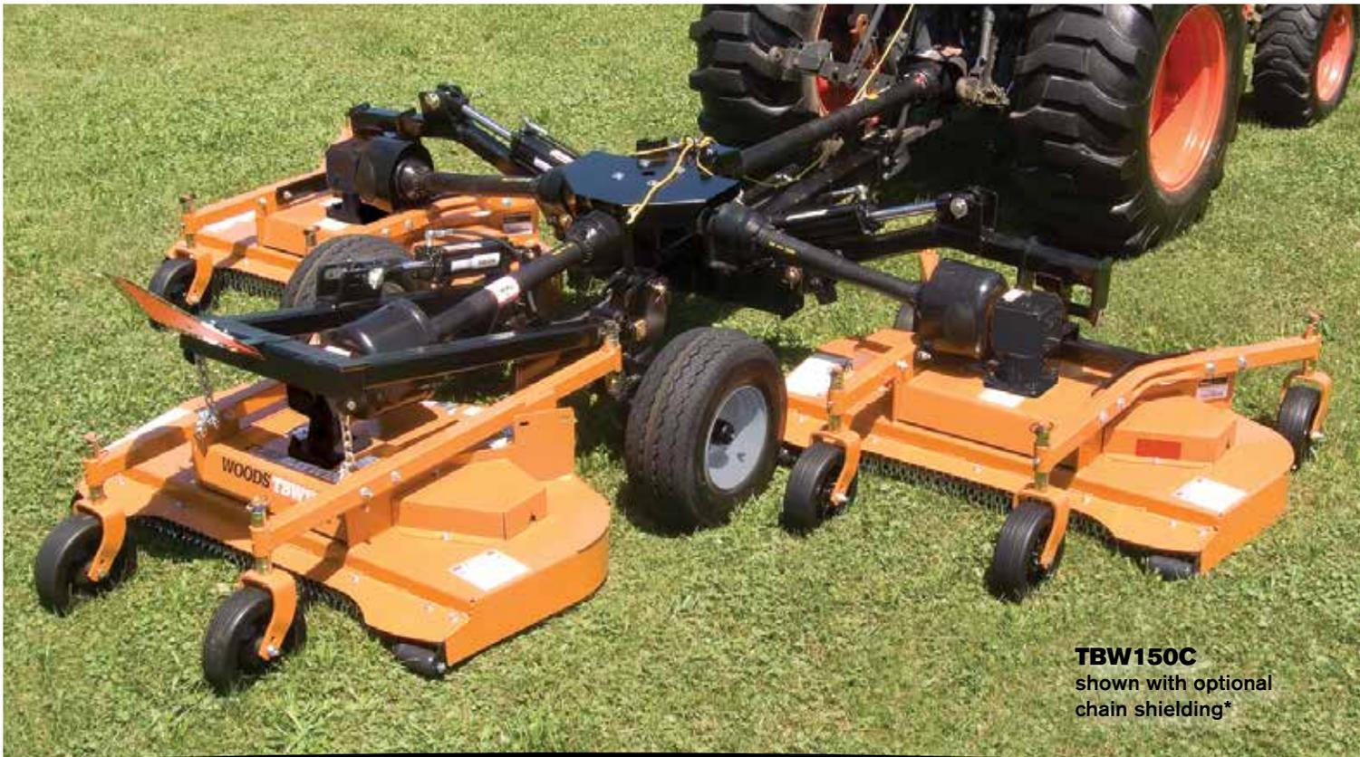
**\*NOTE:** The TBW150C mower passes all applicable safety standards for thrown objects and blade contact. However, if the unit will be used in areas where the possibility of thrown objects could be hazardous to persons or property, it is strongly recommended that optional chain shielding be used for extra protection.
