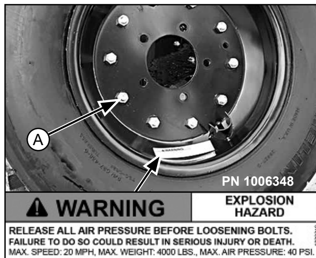
Figure 22. Split Rim Tire Servicing
