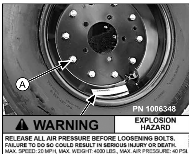
Figure 10. Split Rim Tire Servicing
