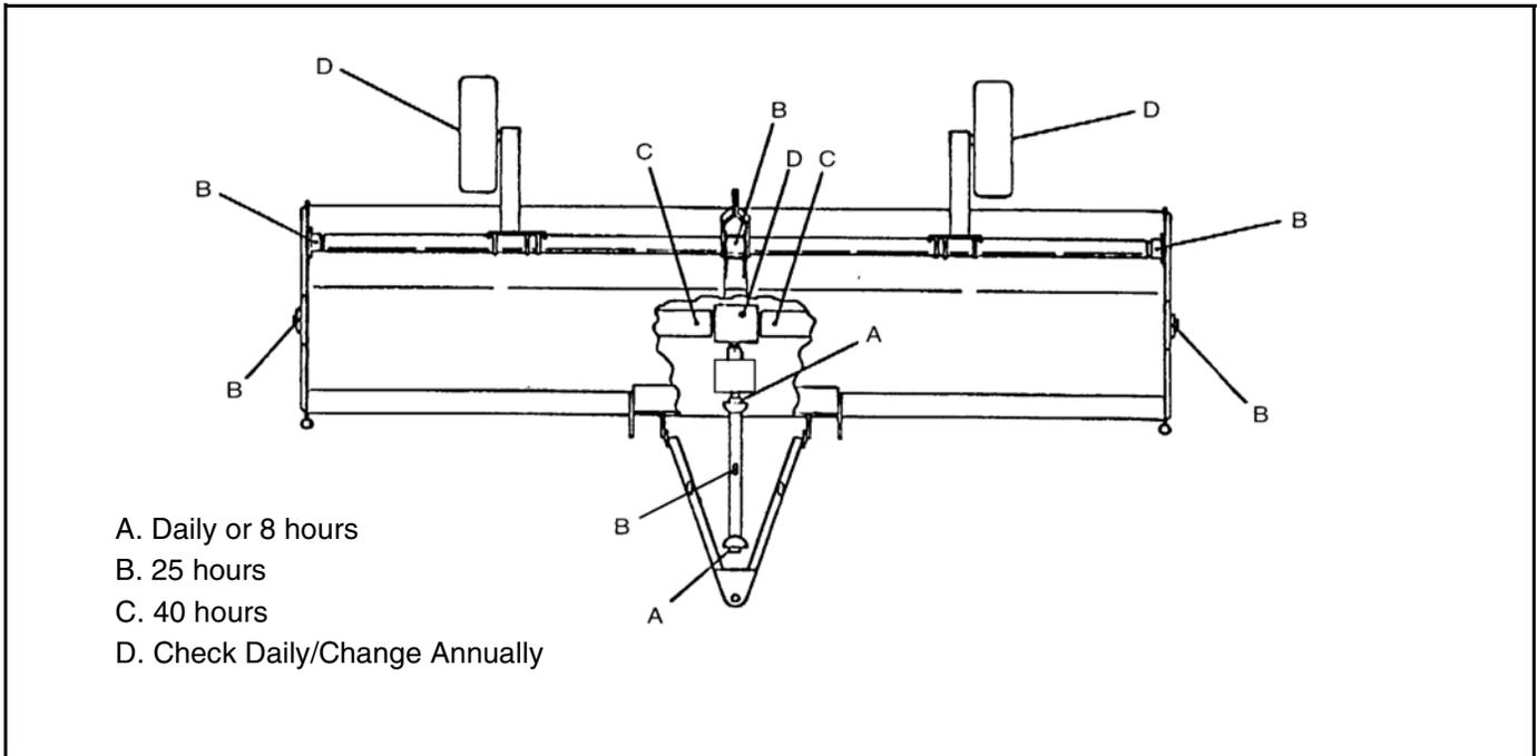
**Figure 26. Lubrication Points**
