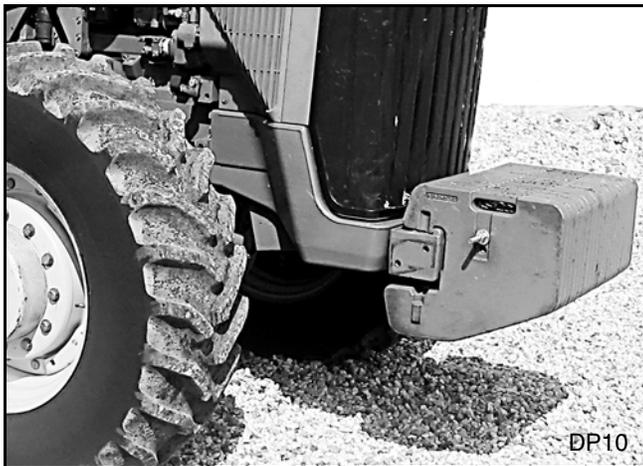
**Figure 2. Tractor Front Weight**
