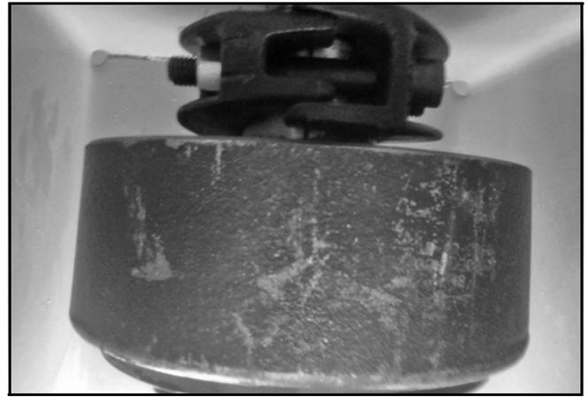
**Figure 44.** Weasler Automatic Clutch (30K)
