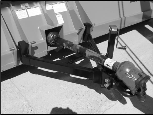
**Figure 51.** Pull-Type Hitch Installed
