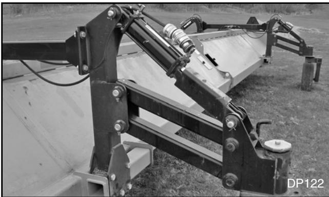
**Figure 48.** Pivot Tubes, Caster Pivots & Cylinders Installed
