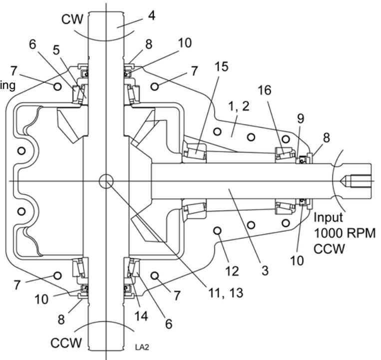
**NOTE:** To separate gearbox halves for servicing, seal guards (8) must be removed first otherwise damage to gearbox housings will occur. Seal guards can be removed by gently prying out of housing with a flat blade screwdriver using the cutout areas machined in the housing to get behind the guards. Use care not to bend guards during removal so they can be reused for reassembly. Replace guards if they are damaged.
