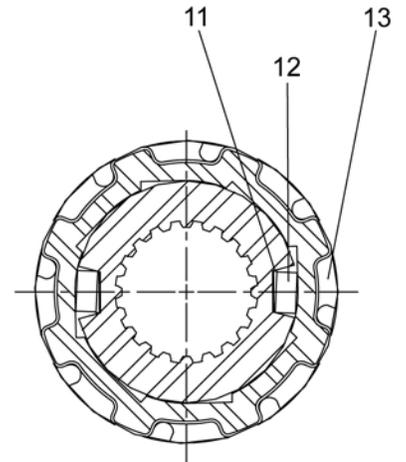
**WEASLER® 30K 3-POINT PTO SHAFT WITH AUTOMATIC CLUTCH (OPTIONAL)
