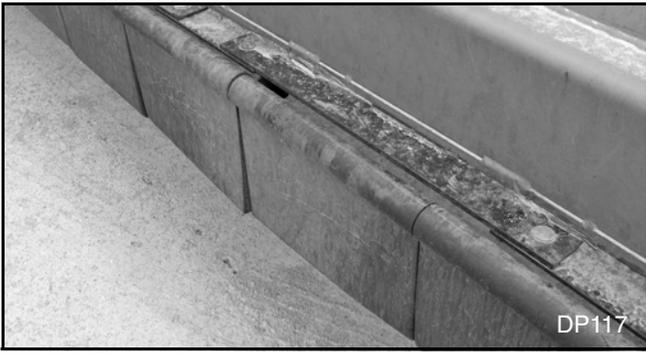
**Figure 39.** Front Rubber Shield Flaps
