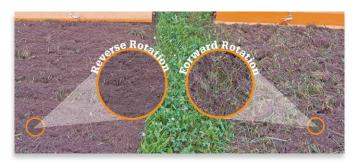
Forward-rotation tillers deliver a finely finished seedbed even in rocky soil conditions. Ideal for low-horsepower tractors.
