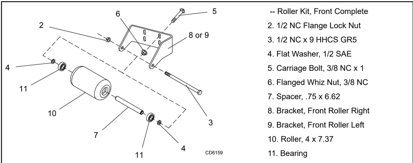
**Figure 32** TBW144 Wing Deck Front Roller Kit Installation
