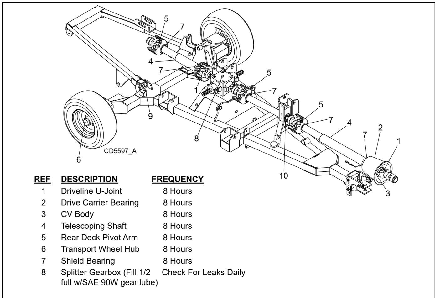
Figure 7. Lubrication Points - Trailer
