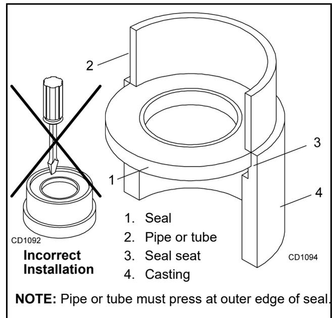
**Figure 18.** Seal Installation
