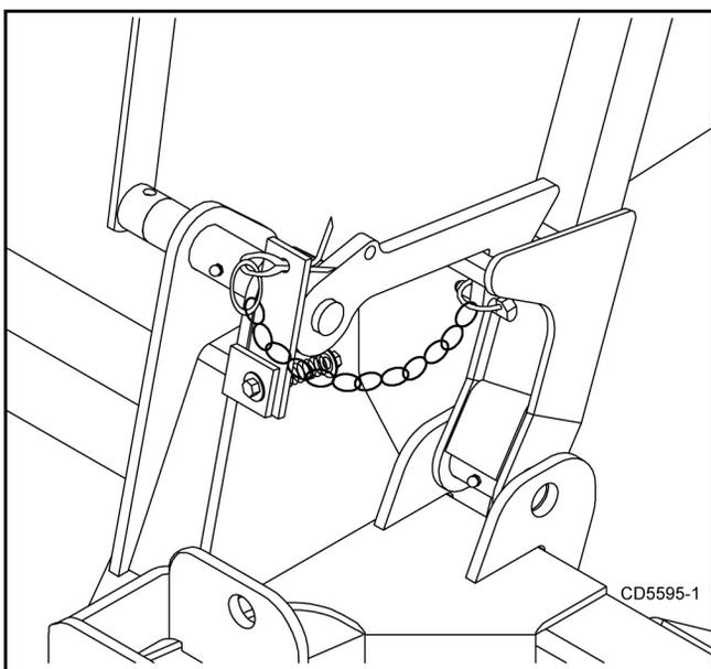
**Figure 5.** Lock Pin Storage Installed (Rear Deck)
