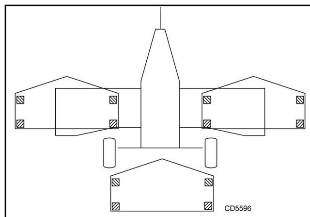
**Figure 6.** Jackstand Placement
