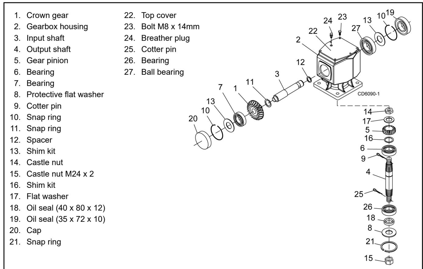
**Figure 19.** Gearbox Assembly
