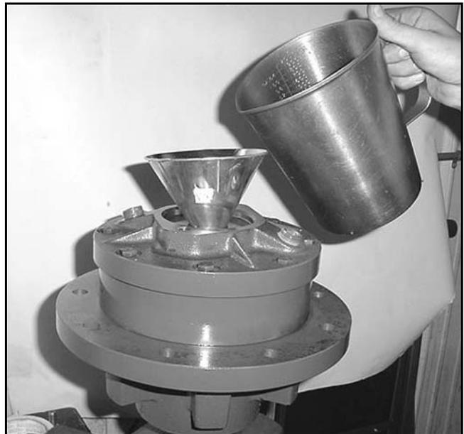
Figure 15. Fill Planetary, Motor Removed
