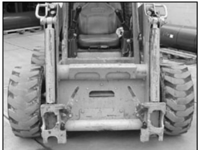
Figure 1. Coupler Latches - Unlocked Position
