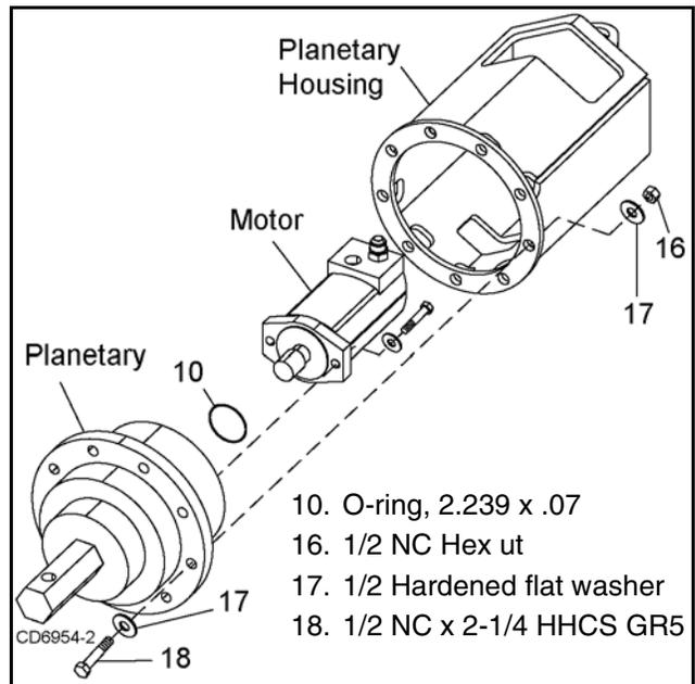
Figure 16. Planetary and Motor Assembly
