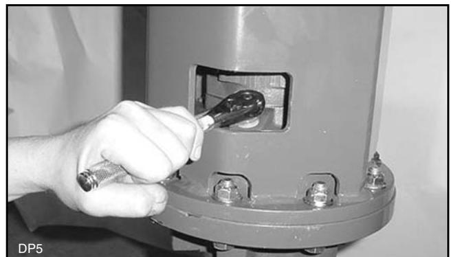
**Figure 6.** Fill Plug Access
