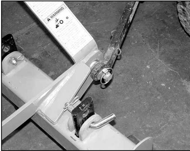
**Figure 1.** 3-Point Lower Lift Arms Connected
