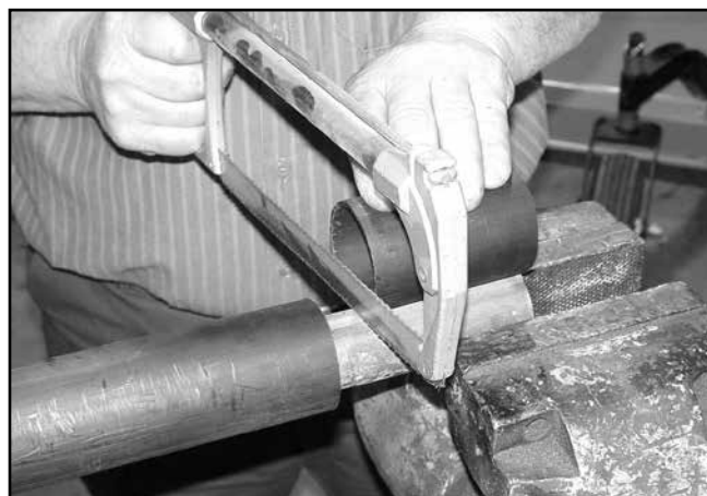
Figure 17. Cut Shaft to Length
