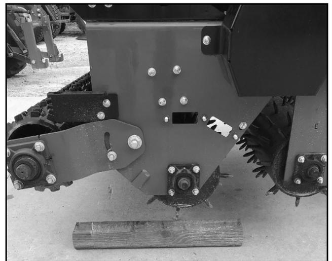
**Figure 7.** Overseeder above Wooden Blocks
