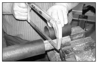
Figure 6. Cut Shaft to Length
