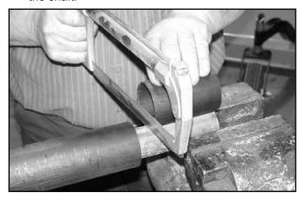
Figure 9. Cut Shaft to Length
