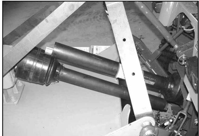
Figure 6. Drive Halves Placed Parallel
