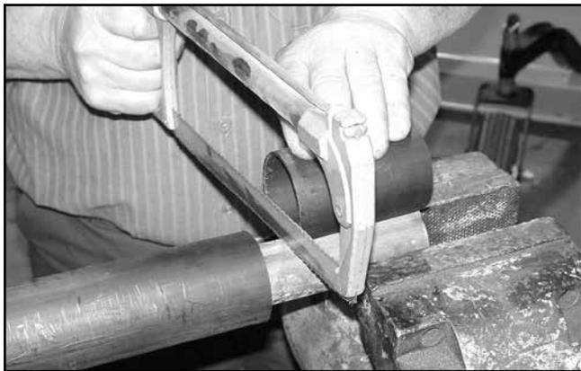
**Figure 9.** Cut Shaft to Length
