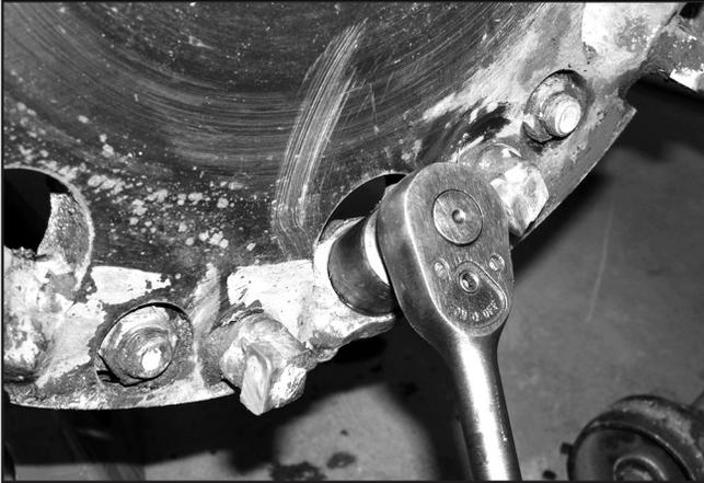
Figure 6. Tooth Installed
