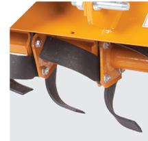
Heat-treated, C-shaped tines penetrate deep, even in thick residue and loose, compacted or rocky soil.
