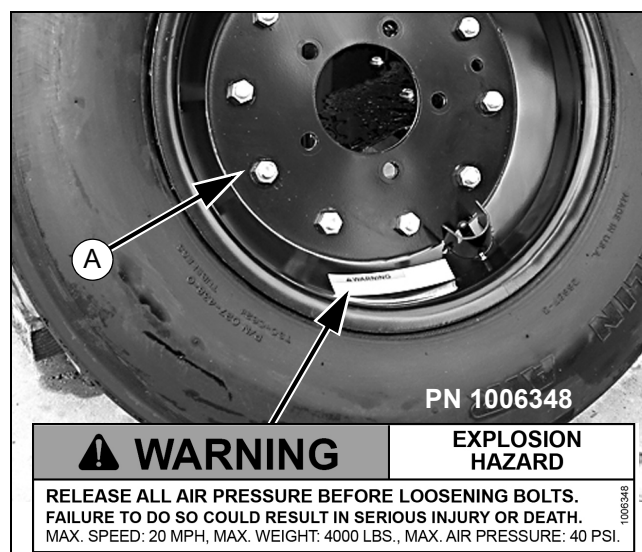
Figure 21. Split Rim Tire Servicing
