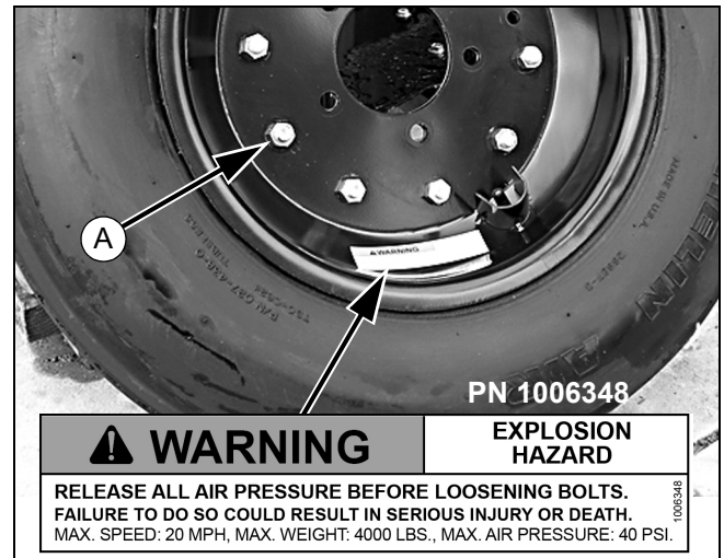
Figure 9. Split Rim Tire Servicing
