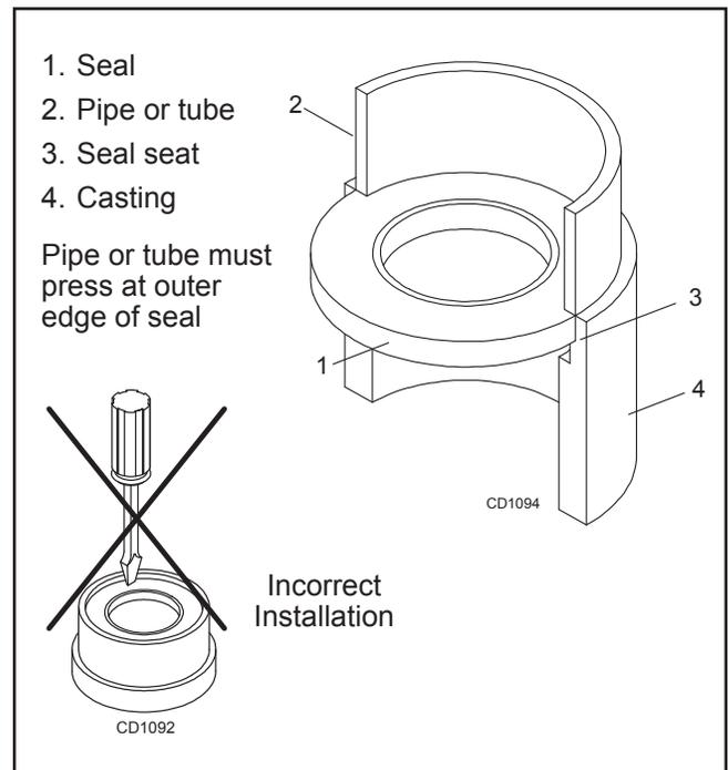
Figure 18. Seal Installation
