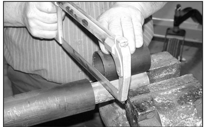
**Figure 8.** Cut Shaft to Length
