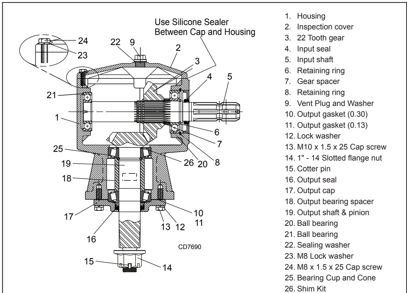
**Figure 19.** DS8.30 Gearbox Assembly
