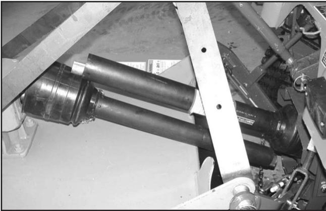
**Figure 5.** Drive Halves Placed Parallel
