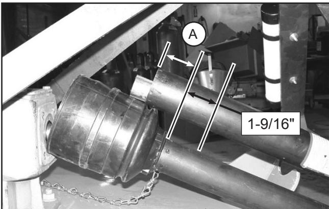
**Figure 6.** Determine Shield Length
