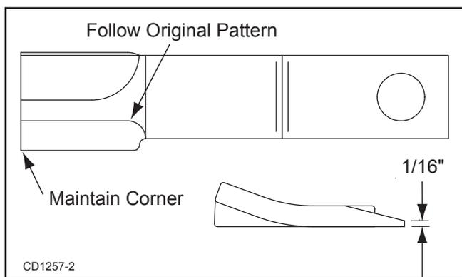
Figure 13. Sharpen Blade Cutting Edge
