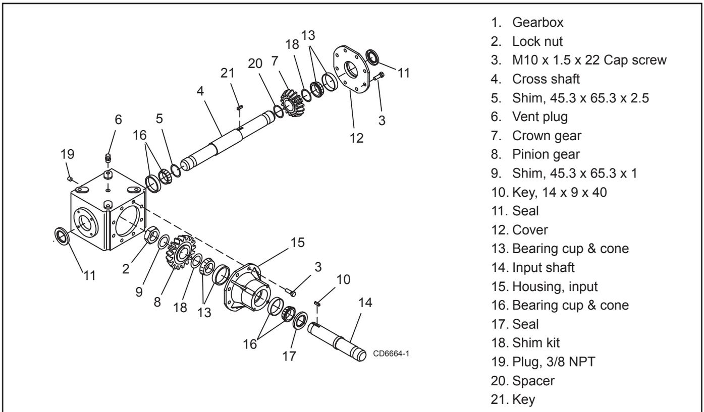
**Figure 21. Center Gearbox Assembly**
