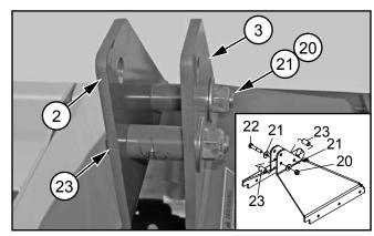
Figure 9. Spacer Sleeve Installation
