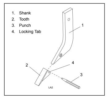
Figure 7. Scarifier Point Replacement
