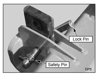
Figure 6. Scarifier Shank Adjustment
