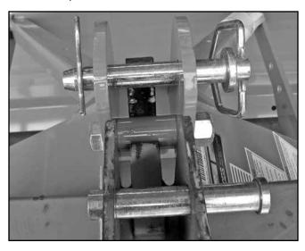
Figure 4. Top Quick Hitch Hook Connection
