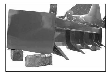
Figure 5. Box Scraper Blocked Up
