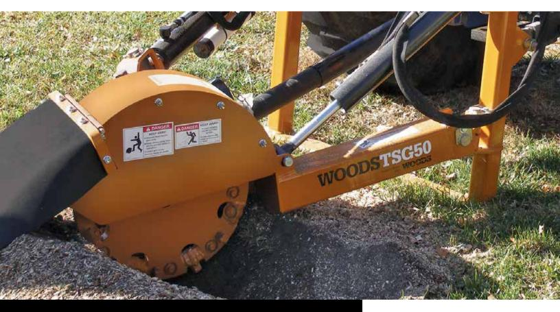
The Woods PTO-powered stump grinders are built to perform — reducing tree stumps to mulch in minutes and grinding below ground level.
