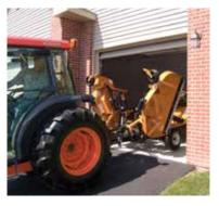
**Folds For Storage** With a folded transport width of only 93 inches the TBW150C can fit into a standard 8-foot garage door.
