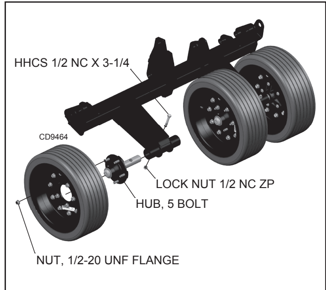
Figure 22. Center Section Wheel and Hub Installation
