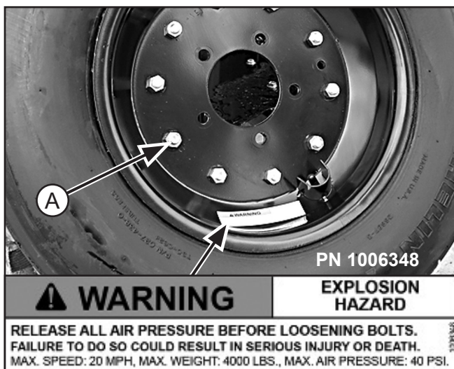
Figure 9. Split Rim Tire Servicing
