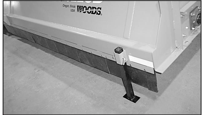
Figure 35. Front Rubber Shield Flaps
