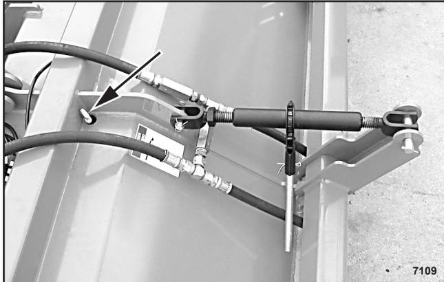
Figure 24. Gearbox Oil Fill Location
