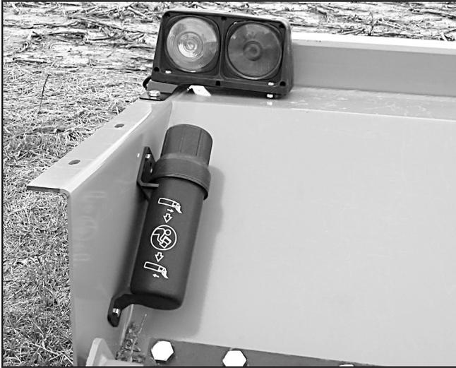
Figure 46. One-Piece Style Manual Tube Installed
