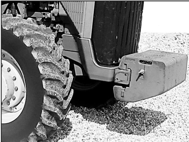
**Figure 2.** Tractor Front Weight
