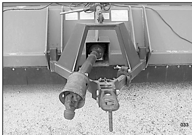
**Figure 45.** Pull-Type Hitch Installed
