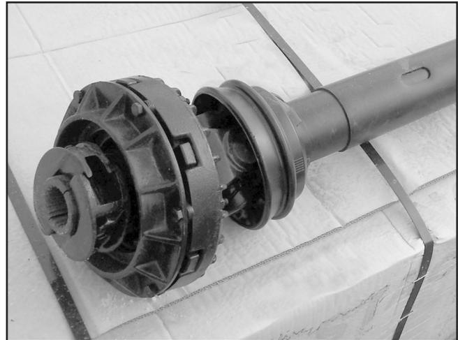
**Figure 39.** Weasler Modular Friction Clutch (24K)
