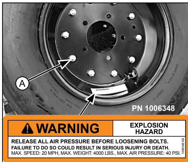
Figure 21. Split Rim Tire Servicing
