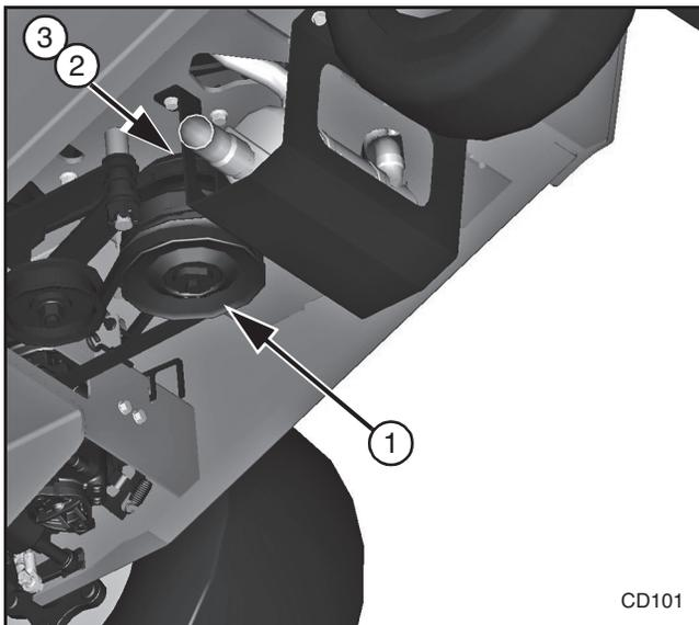
Figure 11. Clutch Assembly
