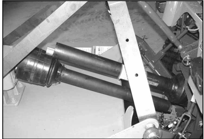
Figure 6. Drive Halves Placed Parallel
