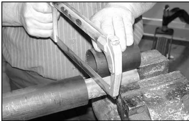
Figure 9. Cut Shaft to Length
