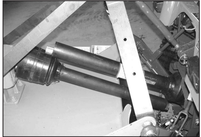
Figure 6. Drive Halves Placed Parallel
